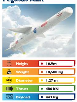
Pegasus ALR, is an air-launched rocket developed by Orbital Sciences Corporation and now built and launched by Northrop Grumman. Capable of carrying small payloads of up 443 kilograms into low earth orbit, Pegasus first flew in 1990 and remains active as of 2019. The vehicle consists of three solid propellant stages and an optional monopropellant fourth stage.
