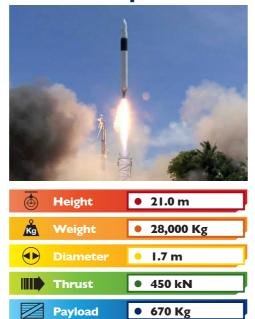
**Falcon I** was an expendable launch system privately developed and manufactured by SpaceX during 2006 - 2009. On September 2008, Falcon I became the first privately-developed liquid-fuel launch vehicle to go into orbit around the Earth. The two stage to orbit rocket used LOX/RPI for both stages, the first powered by a single Merlin engine and the second pwered by a Kestrel engine.
