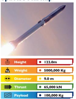
SpaceX Spaceship system is a fully-reusable, two-stage-to-orbit, super heavy-lift launch vehicle under development by SpaceX since 2012, as a self-funded private spaceflight project. The second stage - which is also referred to as 'Starship' is being designed as a long-duration cargo, eventually passenger - carrying spacecraft. It is initially without any booster stage at all to test launch and landing.
