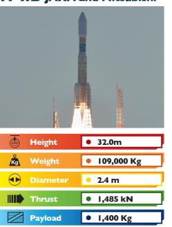
H-IIB JAXA and Mitsubishi was an expendable space launch system jointly developed by the Japanese government's space agency JAXA and Mitsubishi Heavy Industries. It was used to launch the H-II Transfer-Vehicle (HTV or Konotori) cargo spacecraft for the International Space Station. The H-IIB was a liquid-fueled rocket, with solid fuel strap-on boosters and was launched from Tanegashima.
