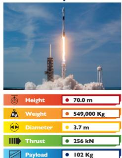
Falcon 9 is a partially reusable two-stage-to-orbit medium-lift launch vehicle designed and manufactured by SpaceX in the United States. It is powered by Merlin-engines, also developed by SpaceX, burning cryogenic liquid oxygen and rocket-grade kerosene (RP-1) as propellants. Its name is derived from the fictional Star Wars spacecraft, the Millenium Falcon, and powered by nine Merlin engines
