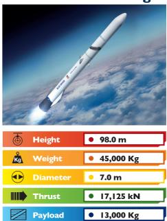
New Glenn named after John Glenn, is a heavy-lift orbital launch vehicle in development by Blue Origin. Design work on the vehicle began in 2012. Illustrations of the vehicle, and the high level specifications, were initially publicly unveiled in September 2016. New Glenn is described as a two-stage rocket with a diameter of 7 metres (23ft). Its first stage will be powered by seven BE-4 engines.
