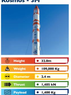
Kosmos - 3M, is a Russian space launch vehicle, member of the Kosmos (rocket family). It is a liquid-fueled two-stage rocket first launched in 1967 and with over 420 successful launches to its name. The Kosmos - 3M uses UDMH fuel and AK271 oxidizer (red fuming nitric acid) to lift roughly 1,400Kg (3000 lb) of payload into orbit.
