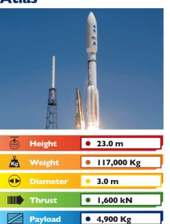
Atlas, is a family of US missiles and space launch vehicles that originated with the SM-65 Atlas. The Atlas intercontinental ballistic missile (ICBM) program was initiated in the late 1950s under the Convair Division of General Dynamics. Atlas was a liquid propellant rocket burning RP-I fuel with liquid oxygen in three engines configured in an unusual 'stage and a half' or 'parallel' staging design.
