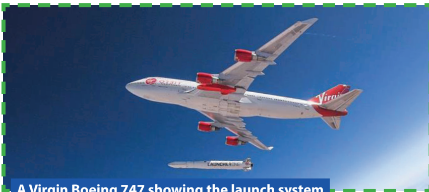
A Virgin Boeing 747 showing the launch system for RAF Project Artemis
