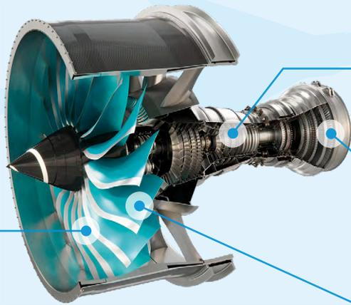
**3 Bang:** Fuel is then added to create a continuous explosion.
