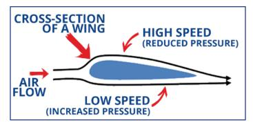
As air flows over a wing the speed of the air and the shape of the wing causes lift and that's how an aircraft gets off the ground.
