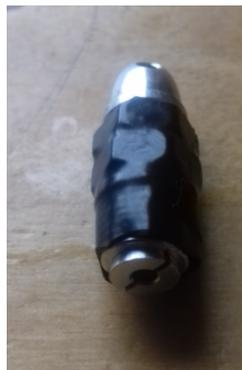
1. Take the dome off the propeller adaptor shaft and add one or two nuts to act as spacers.
